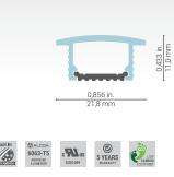
This **profile is made of flexible acrylic with a strip support tab made of aluminum** for better heat dissipation. This outstanding extrusion is recessed with a slight edge on each side. The 5300 profile consists of a built-in lens with edges and a support for the LED strip giving a cabinet, storage or wall lamp.
